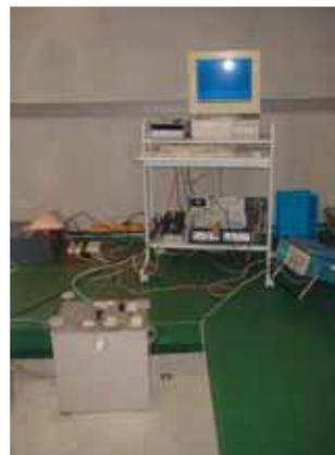
Fig. 2. The ET15 set-up in the Westerbork bunker, in front the gravimeter and in the back its feed-back system.
