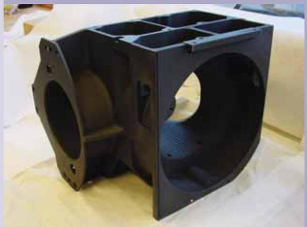
SPIFFI 2k camera housing (upside down) with black coating. In the circular opening at the right the triplet will be mounted. The view through the housing will be closed with the flat mirror. In the circular opening at the left the doublet will be mounted. At the inside there is a rough profile to prevent ghost images.
