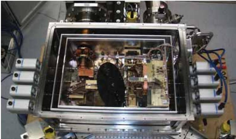
The cold optics installed in the cryogenic chamber as seen from above. The cold-head can be seen top left and the vacuum pump is top right. The cold optics are dominated by the black filter wheel. To both the left and the right of the outer chamber, the eight motors that drive the mechanisms within the cryostat can be seen.
