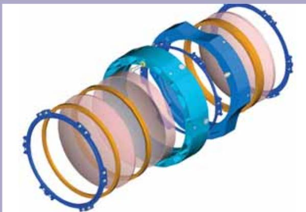
The picture shows the triplet lensmount, with three lenses, two mounts and a few plates and spacers. Typical lens diameter 176 mm.
