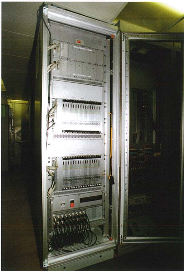
Figure 3.2 The Pulsar Machine (PuMa) in the Faraday cage at the Westerbork Observatory.
