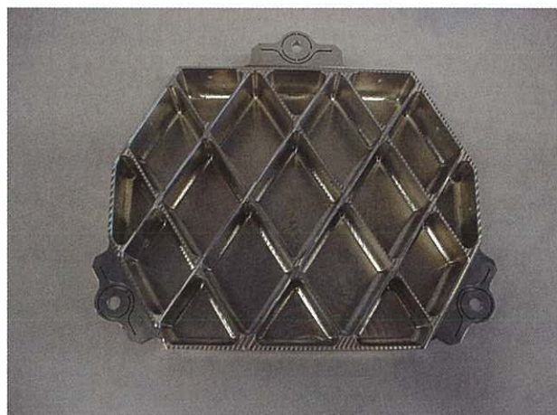
Figure 2.23 One of the mirrors blanks of the TMA collimator/camera system of the High Resolution spectrometer arm. This mirror has a strongly off-axis aspherical surface that will be diamond-cut directly into the Al-6061 blank by Philips Optical Products in Eindhoven (Netherlands). The photo shows the light weighted structure on the back of the mirror. Also shown are the special mounting 'ears' for stress-free isostatic mounting.
