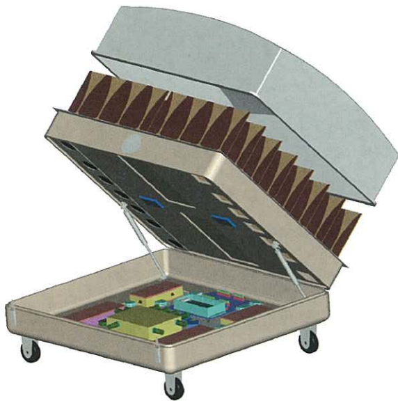
Figure 2.8 (a) Mechanical structure of a tile. The housing is made of low-cost foam. (b) Functional lay-out of a tile. It consists of 64 antenna elements creating two independent beams. Both signals are converted to baseband and digitized with a 40 MHz 12-bit AD convertor.
