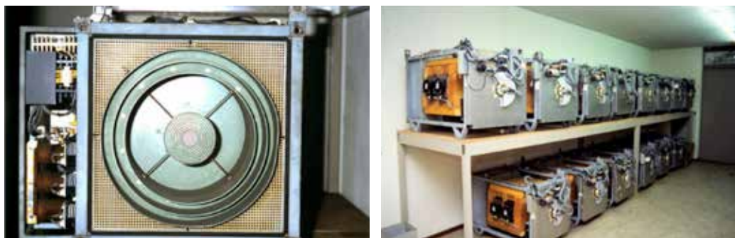
Figure 3 (left): Looking into the 6/50 cm FrontEnd (right): Rack with 15 6/50 cm FE's in Westerbork
