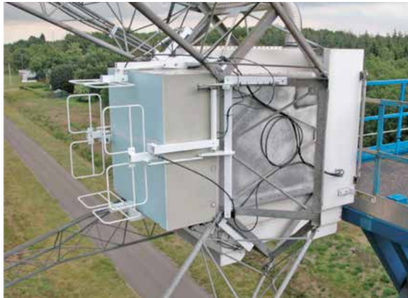
Figure 1: A Low Frequency Frontend mounted on a WSRT dish. The LFFE consists of the white "handrail" style contraptions to the left of the focus box. In this image, they are in their active position. When observing at other frequencies, these are swept out of the way using compressed air.
