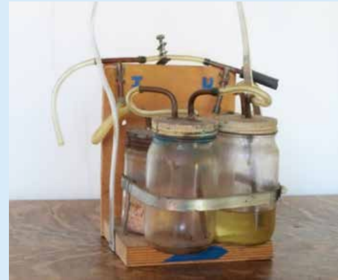
This simple and ultra-sensitive leak detector for the pressurized cables consists of a few jam jars connected by some piping. Gas passing in either direction between two connected pieces of cable bubbles through the silicone oil in the jars. The number of bubbles reflects the gas flow and hence the differential pressure between the two sides. A steady flow betrays a leak.
