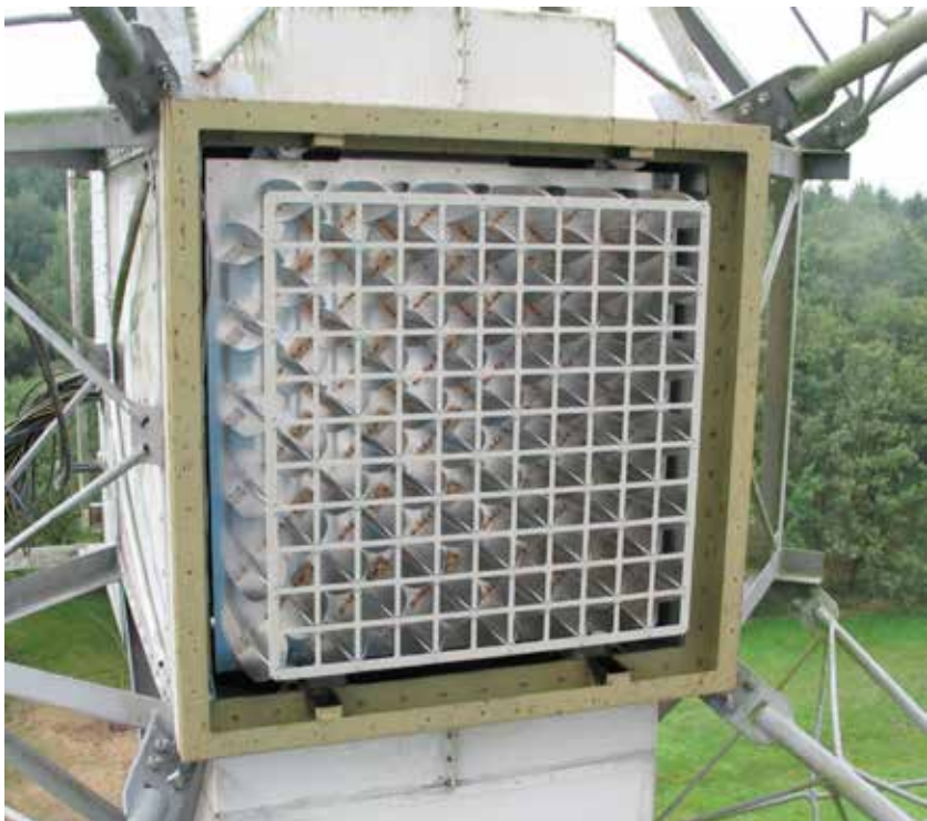
Figure 2 The phased array feed of the Apertif system as mounted in the prime focus box of each WSRT dish.
