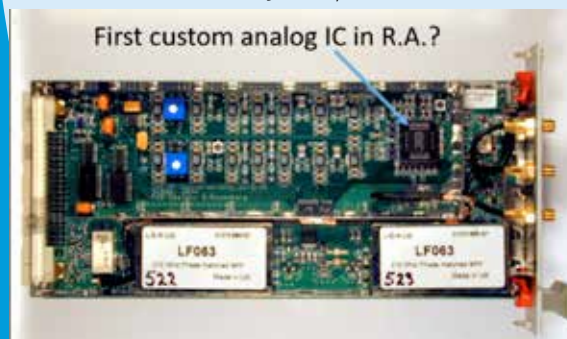
The frequency conversion board including the first analog custom Integrated Circuit in BiCMOS technology designed in collaboration with Catena and produced by Philips in 1997.
