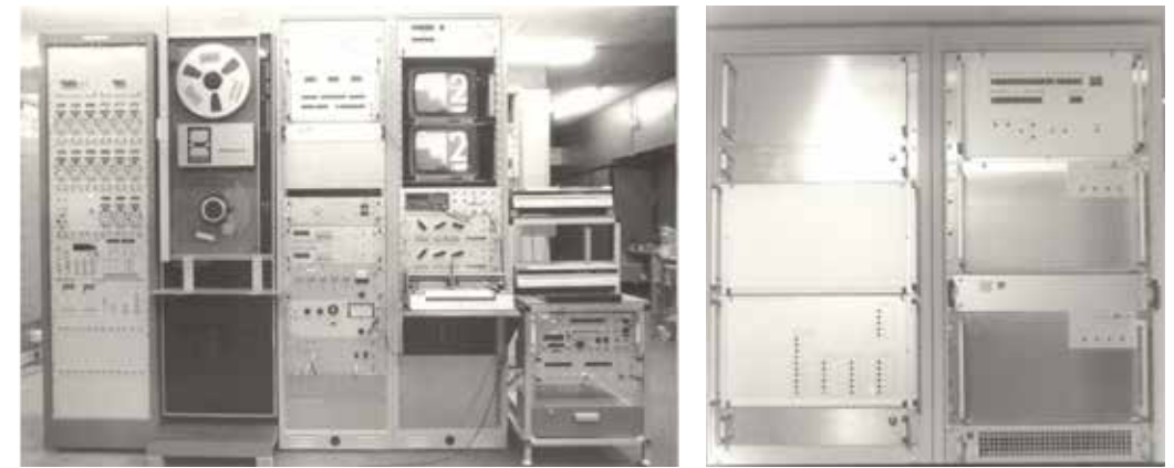
Figure 6. Left: VLBI interface equipment - MKIII tape recorder and electronics system on the left and the WSRT-specific VLBI system on the right. Right: A 1987 picture of the digital adding boxes including fringe rotation which were connected to the DCB (not shown). The digital adder was located inside the RFO shielded cabin. That year, a Hydrogen Maser frequency standard was also installed in Westerbork replacing the Rubidium frequency standard. This allowed the longer integration times essential for 6cm and shorter wavelength observations.
