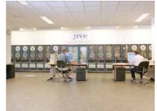
Figure 3. (left) Commissaris Relus ter Beek, with the help of JIVE director Richard Schilizzi, loading a tape on one of the 16 tape drives just before successfully pushing a button to demonstrate fringes from the new data processor. (right) a view of the 16 tape drives and auxiliary electronics and data processor operators.
