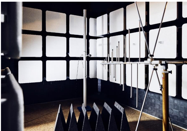
The EMC test room at ASTRON in Dwingeloo (copyright: ASTRON)
