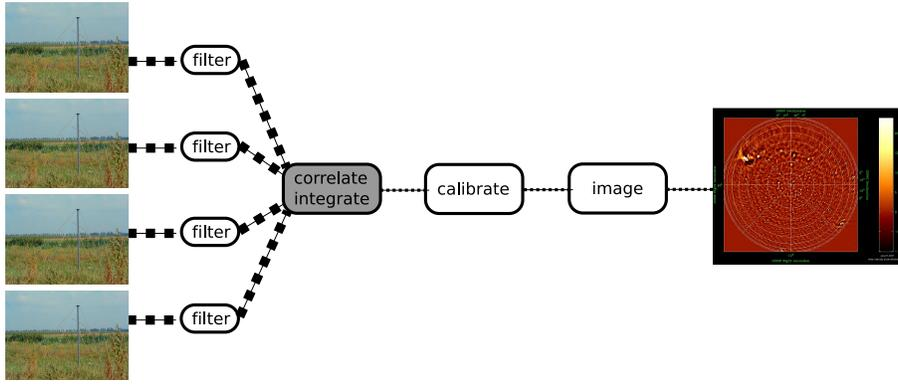
Figure 1: An extremely simplified view of LOFAR processing.
