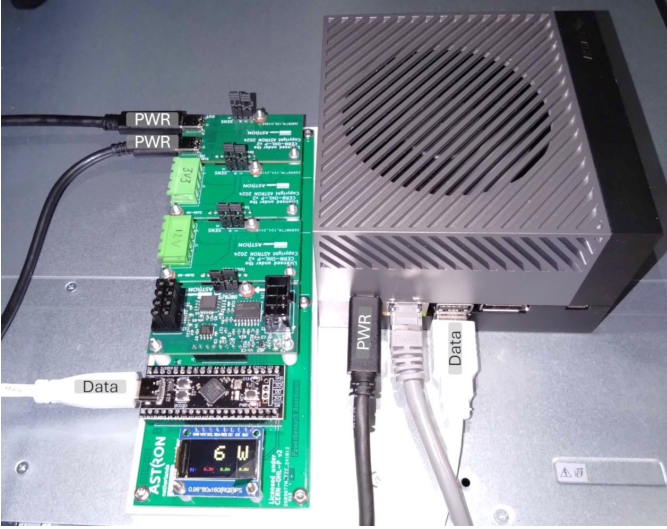
Fig. 9: NVIDIA Jetson AGX Orin with PowerSensor3 on the USB-C power supply, the display shows the idle power.
