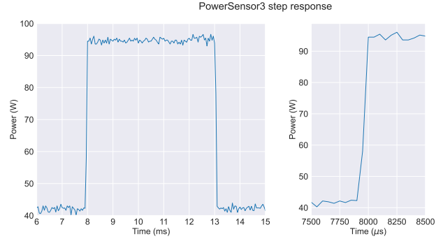
Fig. 5: Step response of PowerSensor3: load stepped from 3.3 A to 8 A plotted in ms scale (left) and \mu s scale (right).
