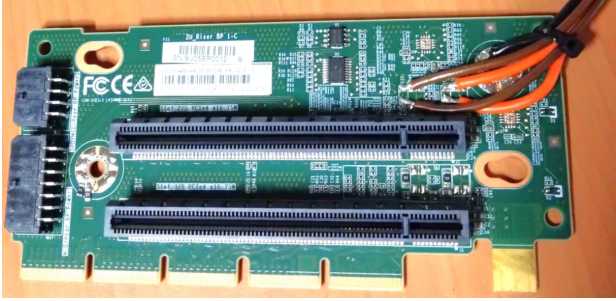
(b) Modified PCIe gen 4 riser card (Lenovo SR665), providing measurement points for 3.3 V and 12 V.
